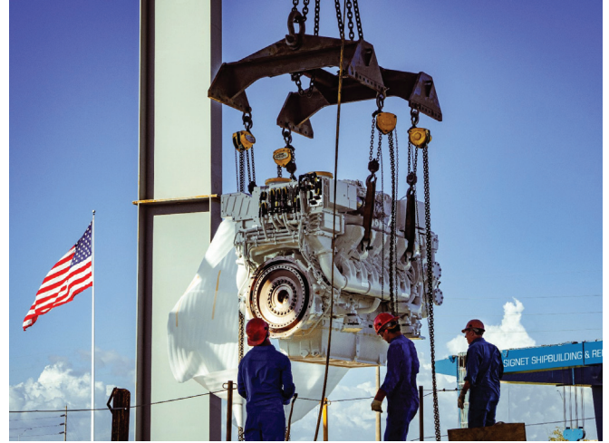
Main propulsion comes from three MTU 12V4000 M65L Tier 4 marine engines producing a total of 7,725 hp.
